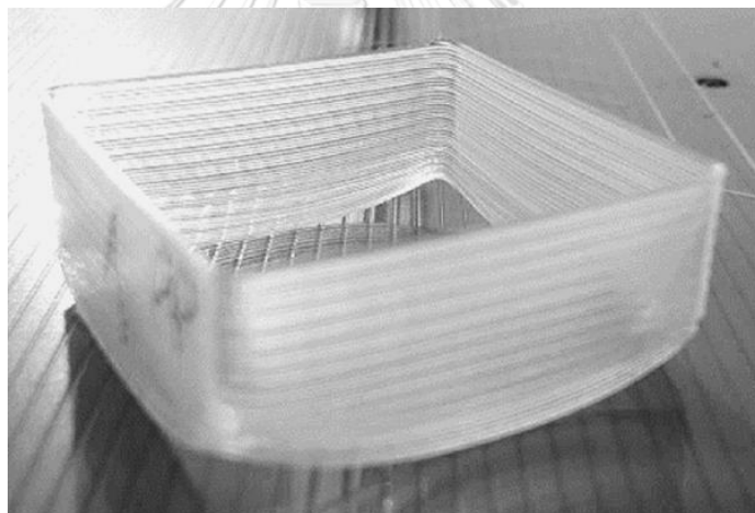
Figure 2.4 The problem of printed PP sample by 3D printing technique [16]
