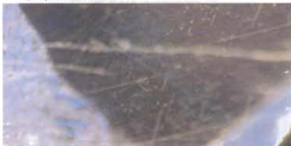
Figure 3.31 Rutile needles oriented 3 directions and intersecting at 60^\circ/120^\circ angles in medium violet sapphire (sample no. MV2, 50X)
