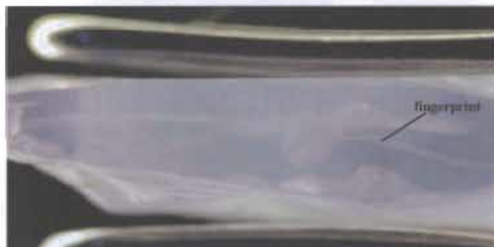
Figure 3.32 White dust which appear milky and fingerprint in medium violet sapphire (sample no. MV5, 20X)
