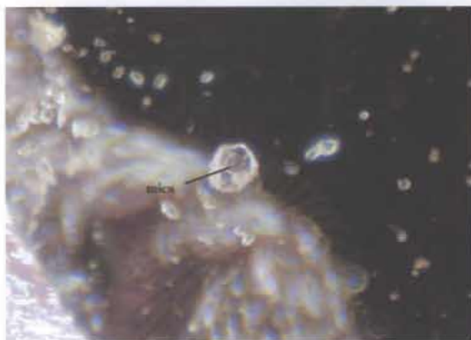
Figure 3.18 Abundant colorless zircon inclusions and a hexagonal platy mica inclusion in light purplish pink sapphire (sample no. LP3, 70X)
