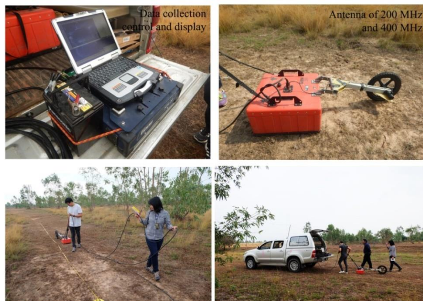
Figure 37 Instruments of GPR including transmitter/receiver as antenna of 200 MHz and 400 MHz and controller/display as a laptop which is operated by SIR-20.
