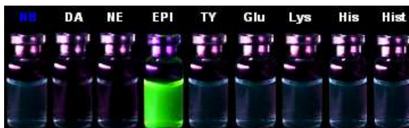
Figure 4.16 Fluorescence color change of sensor NB ( 1 \times 10^{-5} M) in 10% DMSO:phosphate buffer (0.01 M, pH 7.4) in the presence of the various guests 100 equiv.
