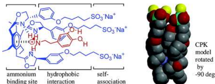
Figure 2.8 Proposed interactions of designed receptor 2 with dopamine•HCl in water and CPK view of an inclusion complex between 2 and dopamine ammonium ion
