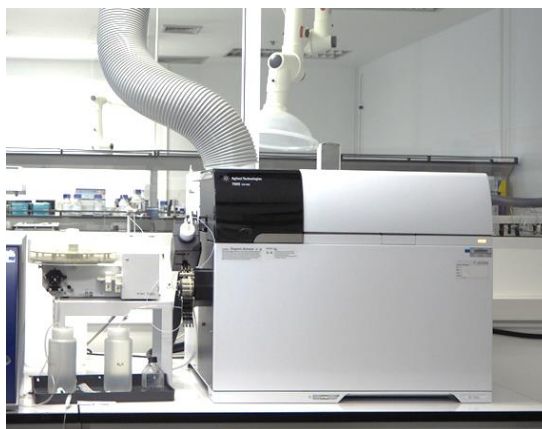
Figure 3.13 Inductively coupled plasma mass spectrometry
