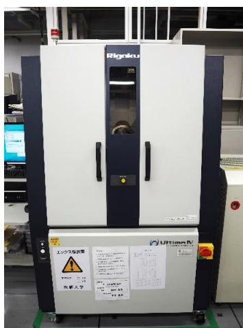
Figure 3.7 X-ray diffraction analyzer
