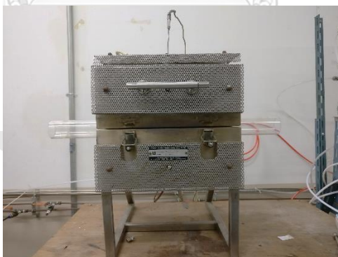
Figure 3.2 Quartz tube reactor
