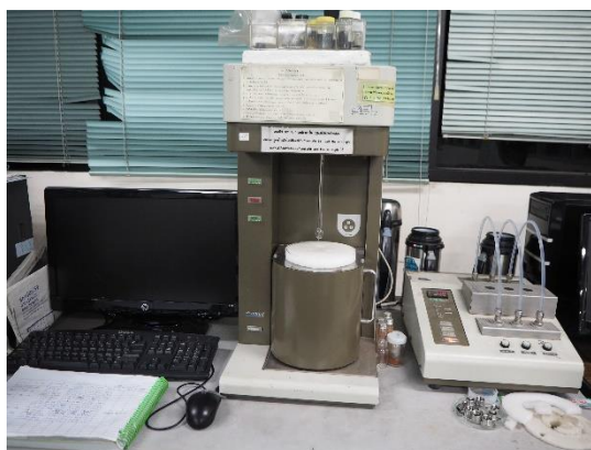
Figure 3.8 N_2 sorption analyzer
