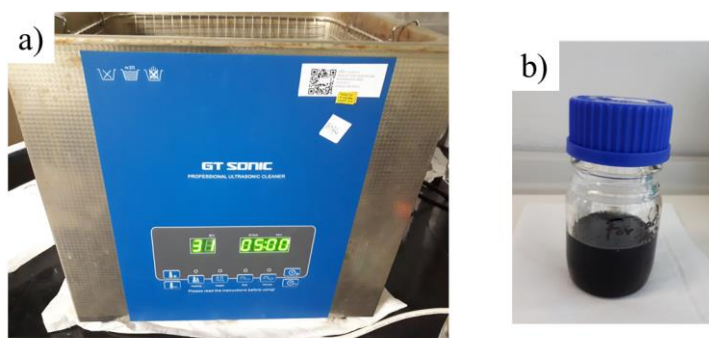
Figure 3.3 a) Ultrasonic bath (GT-2013 QTS, GT SONIC), b) The suspension of CNHs in acid solution
