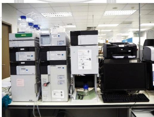
Figure 3.16 High performance liquid chromatography
