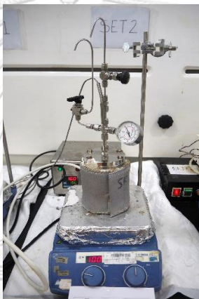
Figure 3.15 In-house batch reactor
