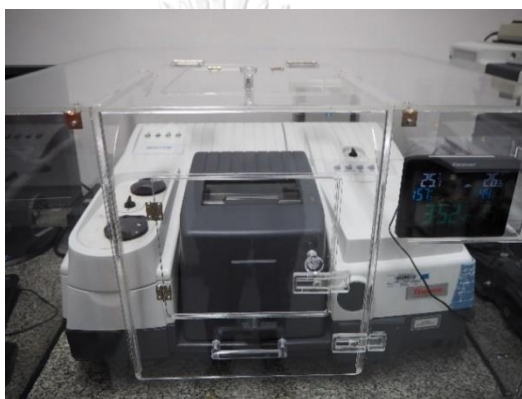
Figure 3.10 Fourier transform infrared (FT-IR) spectrometer
