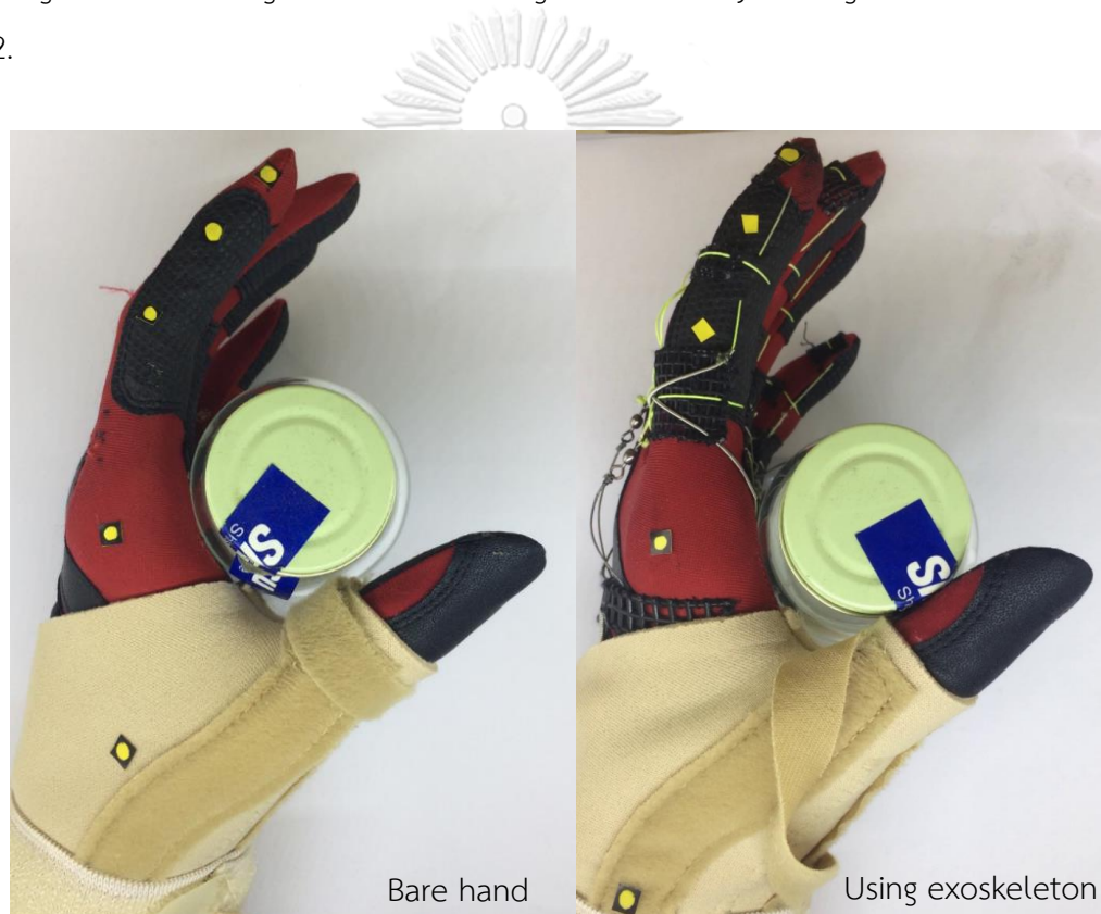
Figure 4.7 Grasping object trajectory evaluation experiment
