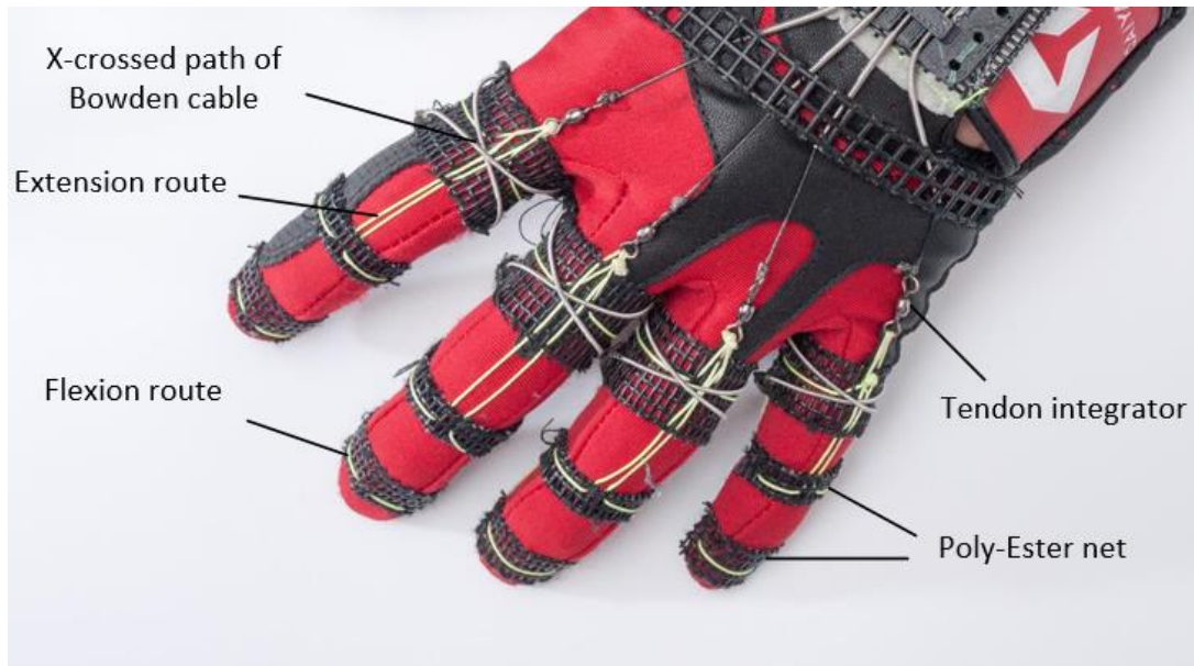
Figure 3.10 Top view of the exoskeleton with flexion and extension tendon routing
