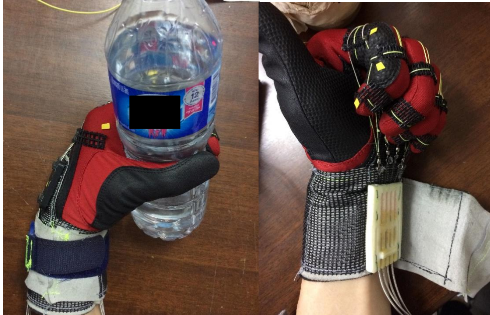
Figure 5.1 (left) Bended wrist when grasping object, (right) Upward Bowden attacher movement
