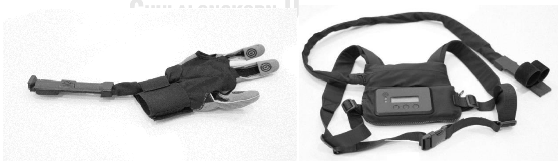
Figure 2.19 (a) the SEM glove and the actuator (left), (b) separately power unit (right), 2012 [28]
