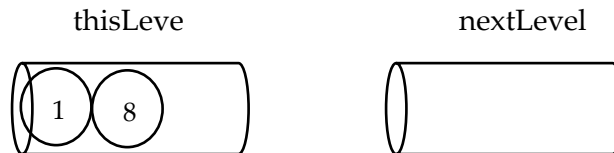
Figure 6-49: Removing all nodes from nextLevel queue and putting them in thisLevel queue.
