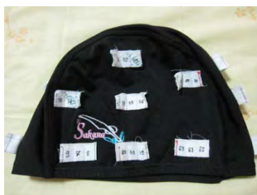
Figure 3.6 The swimming cap, which has small pockets for TLDs to place at suitable locations with high reproducibility.
