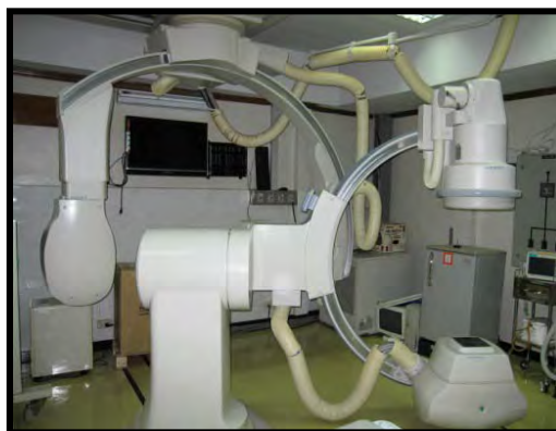
Figure 3.1 DSA equipment systems with bi-plane.
