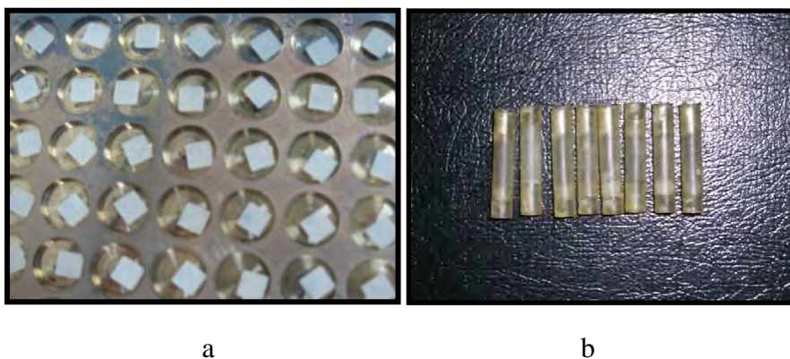
Figure 3.2 Thermoluminescent dosimeter (TLD 100) was the lithium fluoride (LiF) crystal doped with magnesium and titanium (LiF:Mg,Ti). (a) TLD chips with the dimension of 3.2 \times 3.2 \times 0.89 \text{ mm}^3 and (b) tube of TLD chips.
