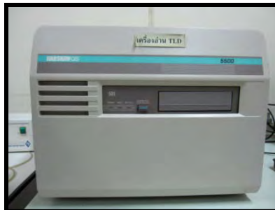
Figure 3.3 The Harshaw model 5500 automatic thermoluminescent dosimeter reader.
