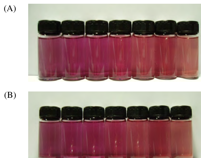
Figure 11 Appearance of TK-AuNPs in varying weight ratios of Au to TK fucoidan; 1:5, 1:10, 1:20, 1:30, 1:40, 1:50 and 1:60 (from left to right) after synthesis (A) and one month storage (B)
