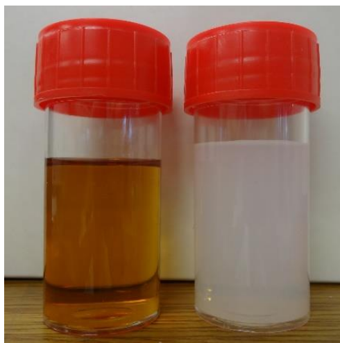
Figure 2.1 Castrol Cooledge BI cutting oil (left) and the 1 g/L cutting oil emulsion (right)
