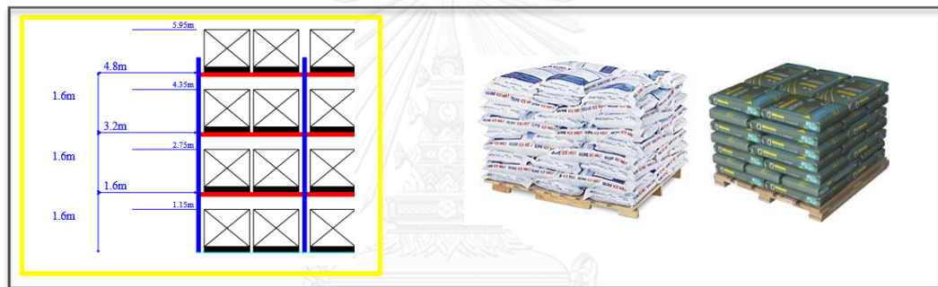
Figure 4-27 : Zone A, B and E Rack – Powder bag storage (palletized) and rubber storage
