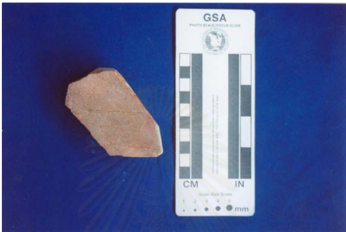
Figure 2.10. Reddish-brown arkosic sandstone of Lam Thap Formation. Grid reference 282858, Cross-section 1.
