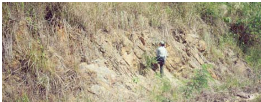
Figure 3.13. Calcareous siltstone of Sai Bon Formation illustrates the west dipping bedding planes. Grid reference 197330, Cross-section 2, View toward the southeast.
