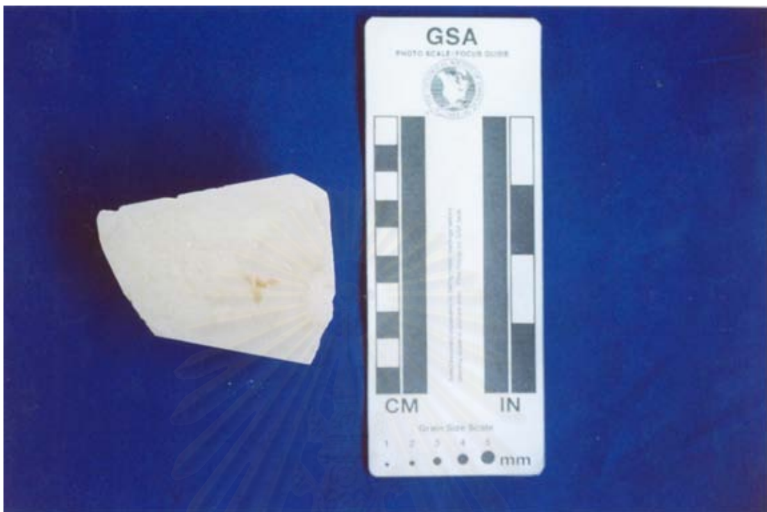
Figure 2.4. Light gray calcareous sandstone of Sai Bon Formation. Grid reference 907730, Cross-section 3.
