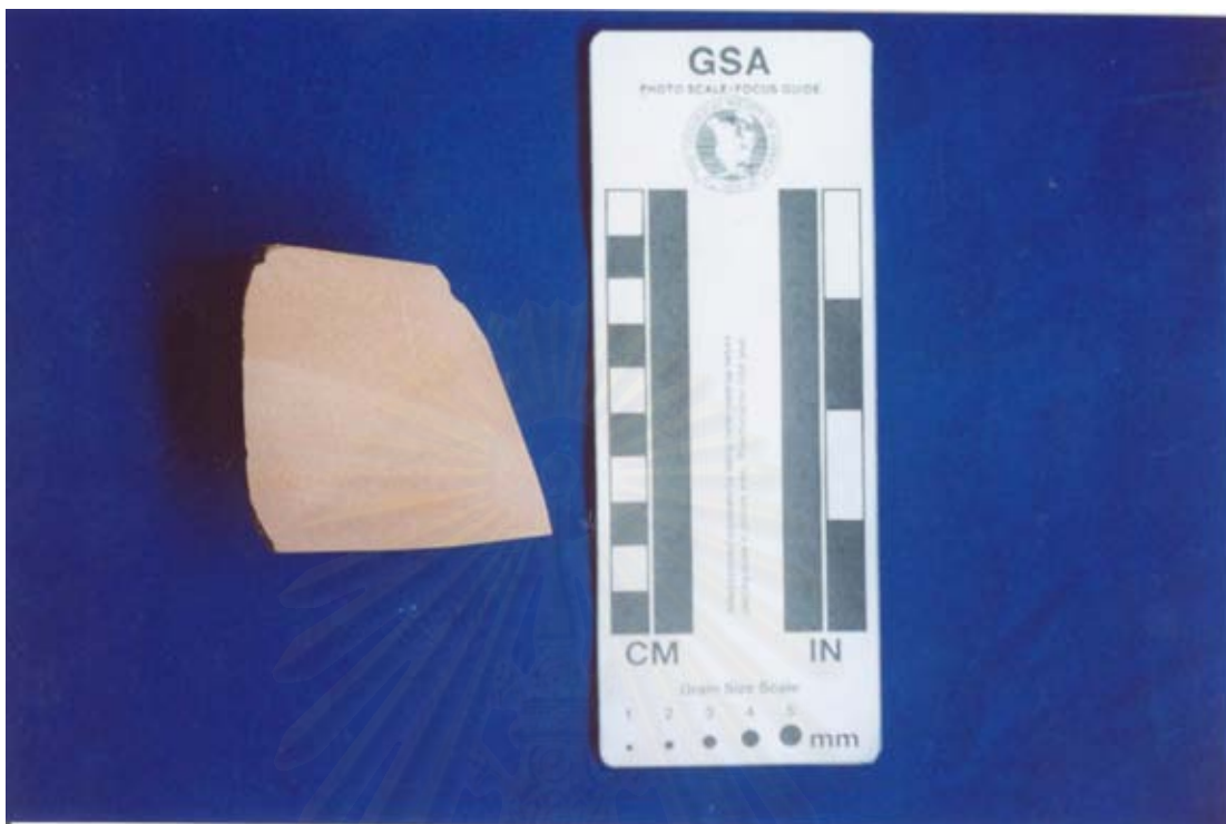
Figure 2.12. Yellowish-brown arkosic sandstone of Lam Thap Formation. Grid reference 204274, Cross-section 2.
