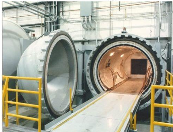
Figure 2.8 The autoclave used in the laminate fabrication process [4] .
