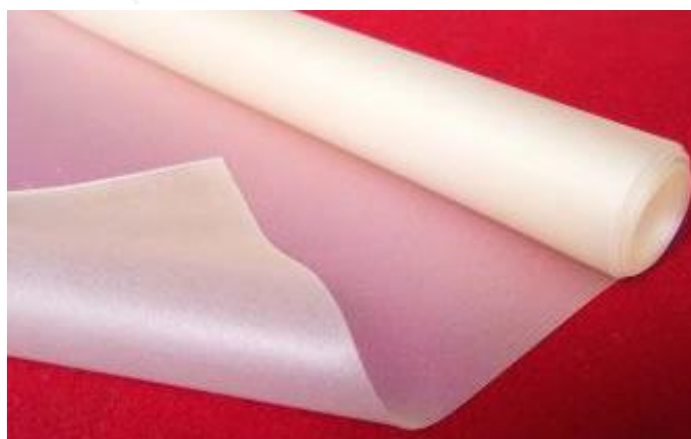
Figure 2.4 Example of Polyvinyl butyral (PVB) film [17] .
