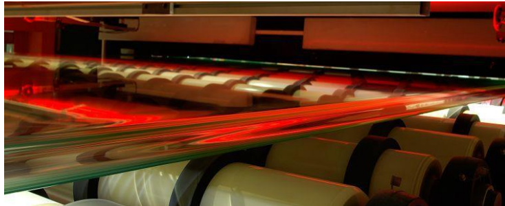
Figure 2.7 The rolling machine in the pre-nip and de-airing process [4] .
