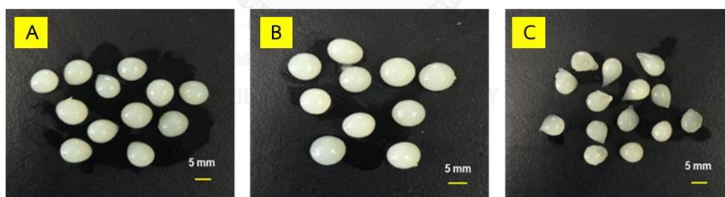
Figure 4.9 Effect of sodium hydroxide concentration (A) 5, (B) 10 and (C) 15% (w/v) on bead formation for controlled release saponin
