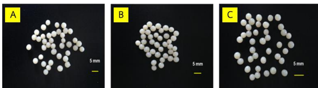
Figure 4.8 Effect of TPP concentration (A) 1, (B) 3 and (C) 5% (w/v) on bead formation for controlled release saponin
