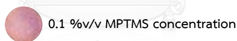
Figure 4.4 The color of AgNPLs paper coated with 0.1 %v/v MPTMS and 200 ppm AgNPLs.
