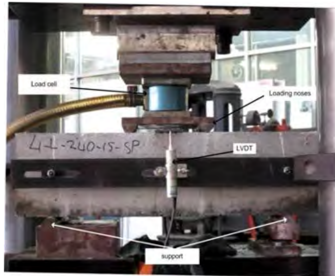
Figure 3.20 Installing the LVDT and load cell
