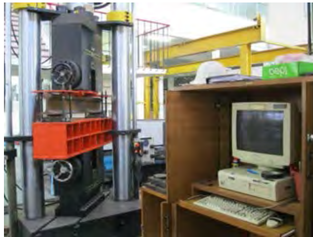
Figure 3.7 Instron (Model no. DYNS, Serial no. H 2029, 1000-kN capacity)
