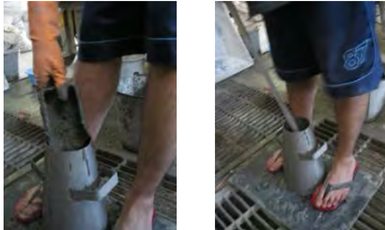
Figure 3.15 Slump test procedure
