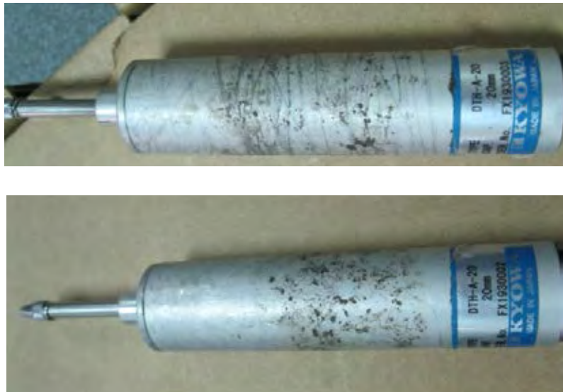
Figure 3.10 Kyowa LVDTs (Model DTH-A-20, Serial no. 1930002 and 1930003, 20-mm rated capacity)
