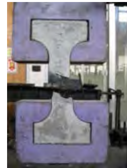
Figure 3.25 Installing briquettes and the briquette after tensile testing
