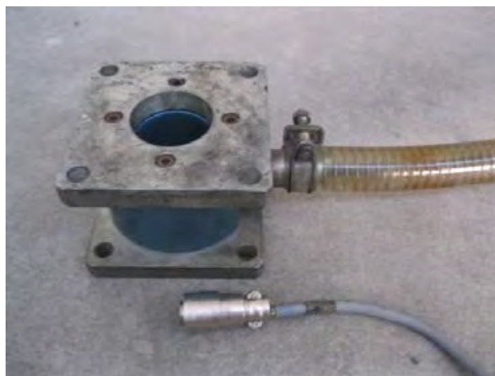
Figure 3.9 Kyowa Hollowed Load Cell (Model BL-10TB, Serial no. AU1170, 10-ton capacity)
