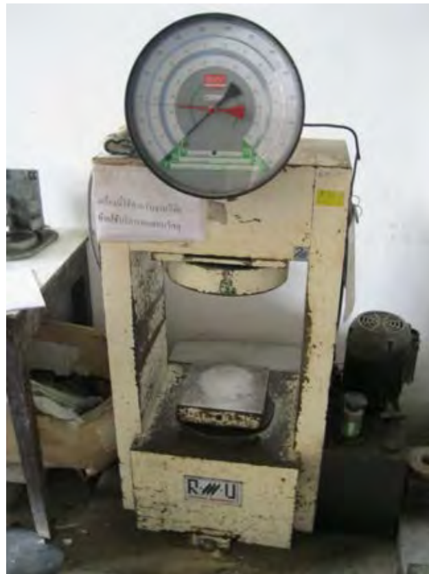
Figure 3.6 RMU Compression Testing machine (serial 85, 3000 kN capacity)
