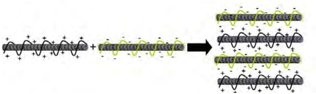
Figure 4.59 Schematic mechanism of layer-by-layer self assembly of (MWCNTs.PDADMAC) / (MWCNTs.PANi.PSS) multilayer thin films
