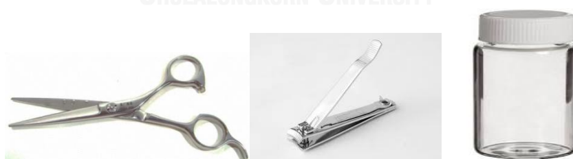
Figure 3. 5 Sampling equipment: stainless steel hair scissors, stainless steel nail clipper, and glass bottle
