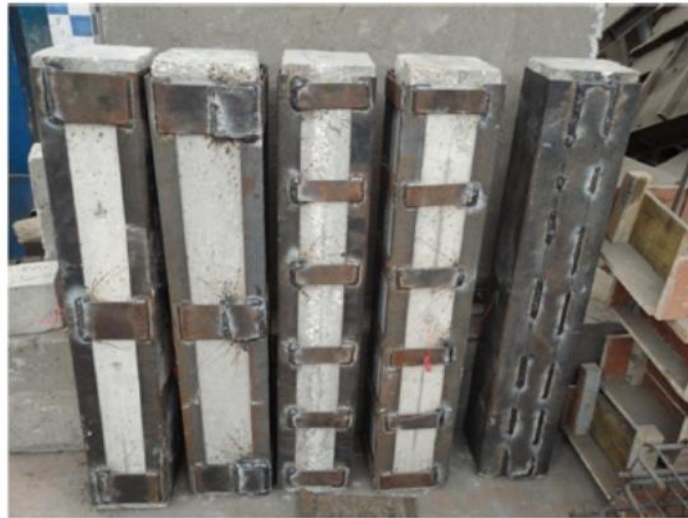
Figure 2.22 Strengthened specimens after casting and jacket erection
