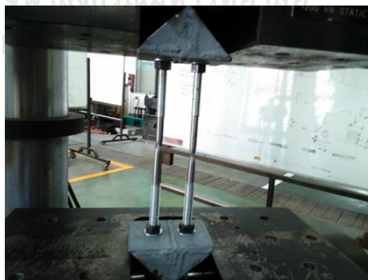
Figure 3.6. Final condition of the steel rod
