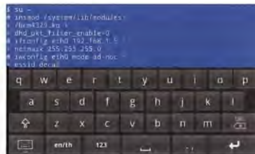
Figure 5. Setting up wireless Ad Hoc network on Android
