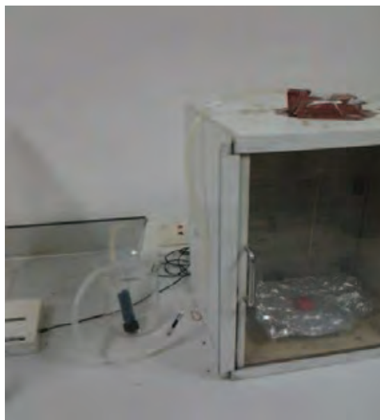
Figure 3.8 The chamber test of incense smoke
