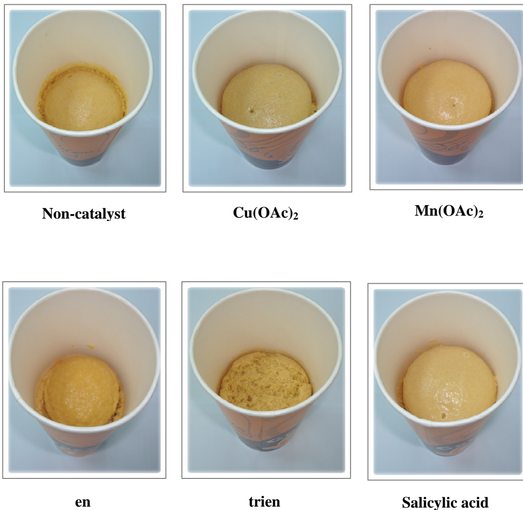
Figure 4.34 External appearance of RPUR foams catalyzed by metal acetates, amines and salicylic acid
