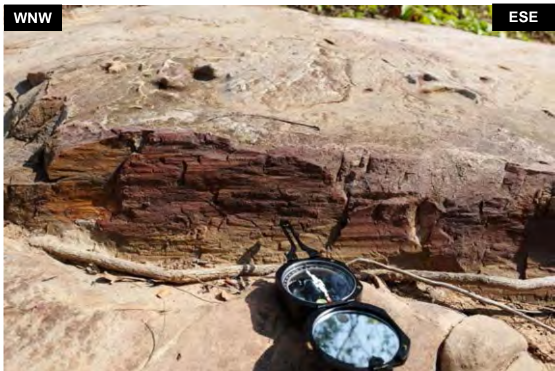
Figure 4.12 WNW-ESE trending dextral strike-slip fracture in Thep Phana waterfall showing slickensides along fracture plane.
