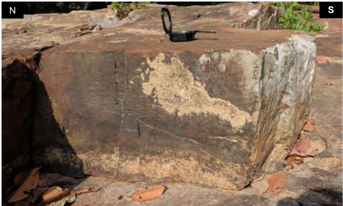
Figure 4.20 N-S trending open fracture in Thep Phana waterfall showing no evidence for movement along fracture plane.
