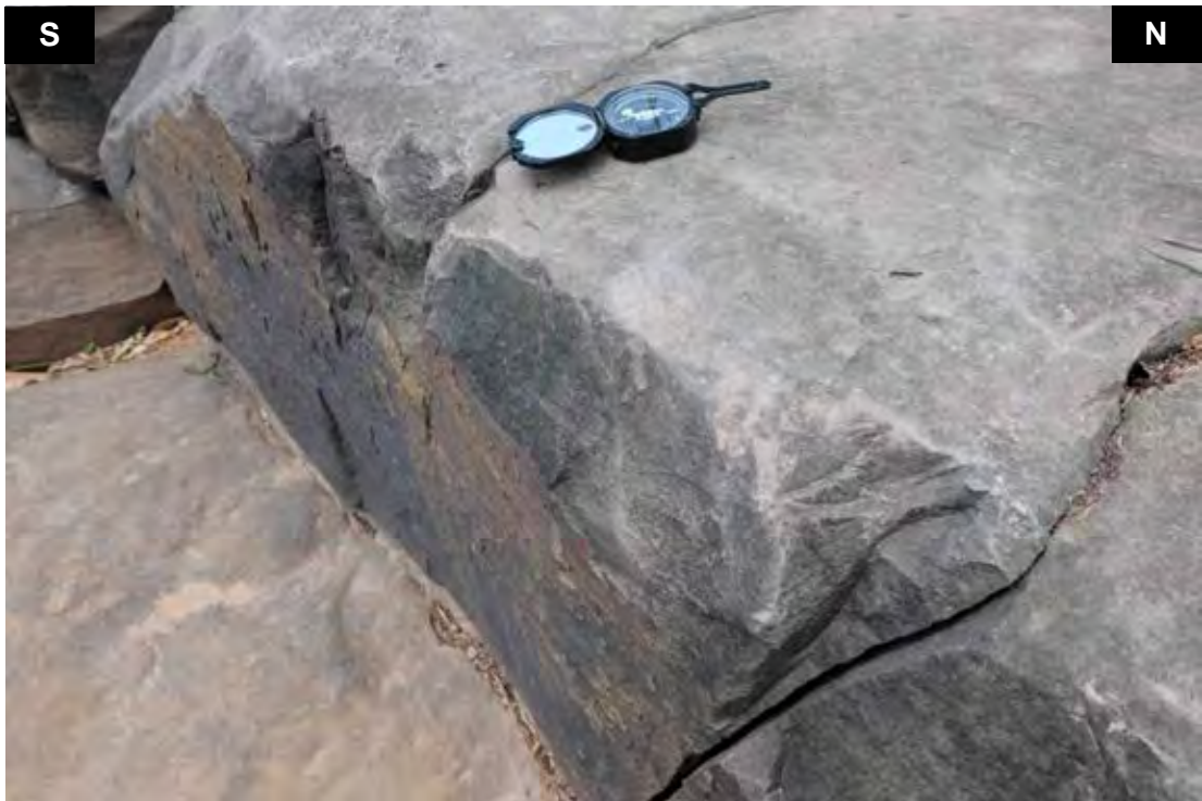
Figure 4.17 ENE-WSW trending sinistral strike-slip fracture in Wat Nam Tok Charoen Tham showing slickensides along fracture plane.
