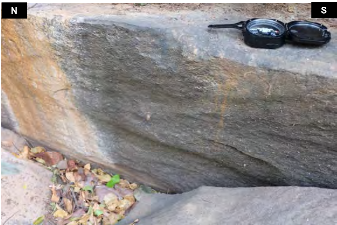
Figure 4.22 N-S trending open fracture in Wat Nam Tok Charoen Tham showing no evidence for movement along fracture plane.
