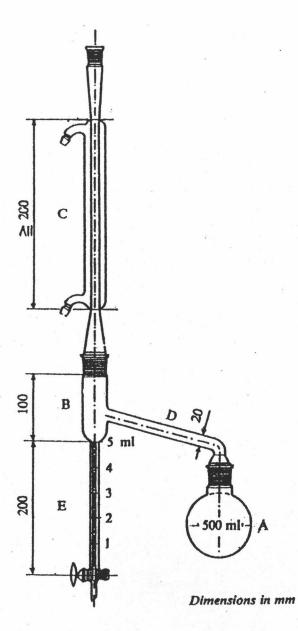
Figure 12 Apparatus for moisture content determination.
