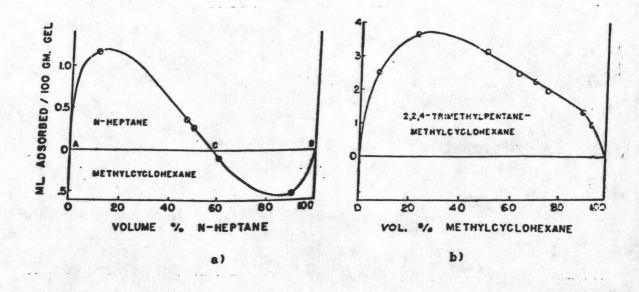
Figure 1.2 Adsorption isotherms neglecting volume in the liquid mixture as a result of solute adsorption, a) S-type isotherm.
