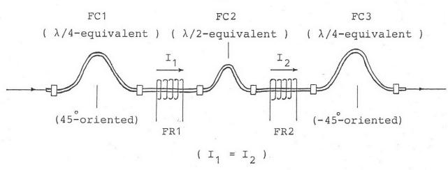
Fig. 57. Principle idea of an electronically controllable phase shifter. FR: Faraday rotator; FC: fiber crank.
