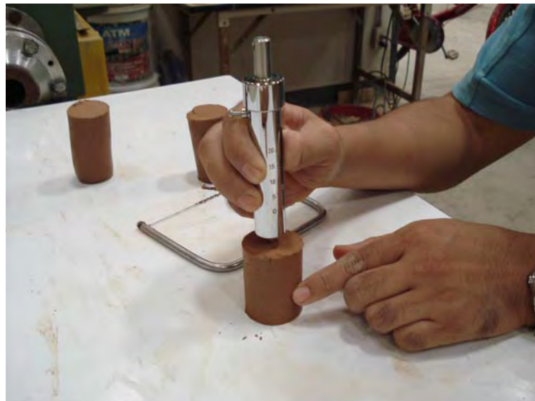
Fig. 3.7 Picture of measuring method for controlling hardness of the clay dough
