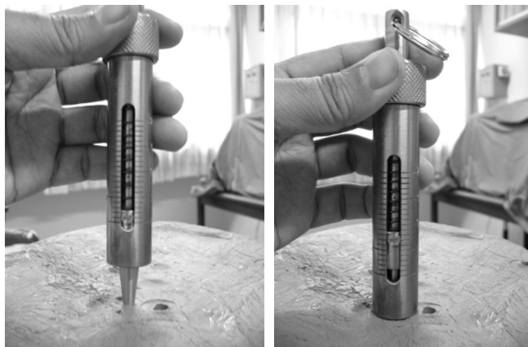
Fig. 3.4 Photographs illustrating the measurement method of the hardness tester
