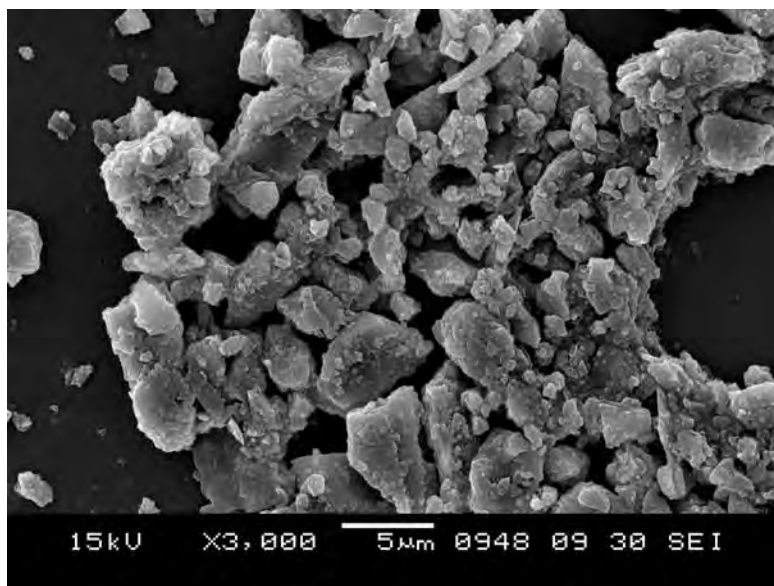
Fig. 4.7 SEM micrograph of pottery stone
