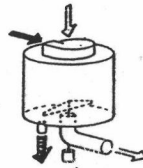
Co-current, flat base, with rotary atomizer, for special products. Also suitable for spray cooling.
