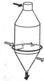
Mixed flow, with nozzle atomizer, for ceramic products.
