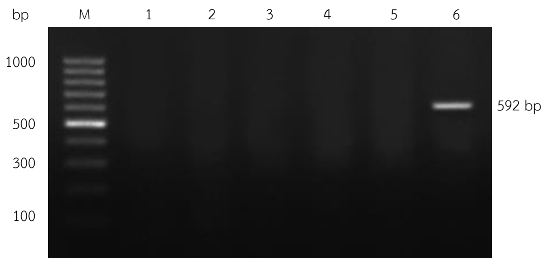
Figure 17: Electrophoresis of PCR products for the screening of integrative and conjugative elements (ICEs). Lane M, 100 bp marker; Lane 1-5, int SXT -negative V. parahaemolyticus isolates; Lane 6, a positive control for SXT integrase gene
