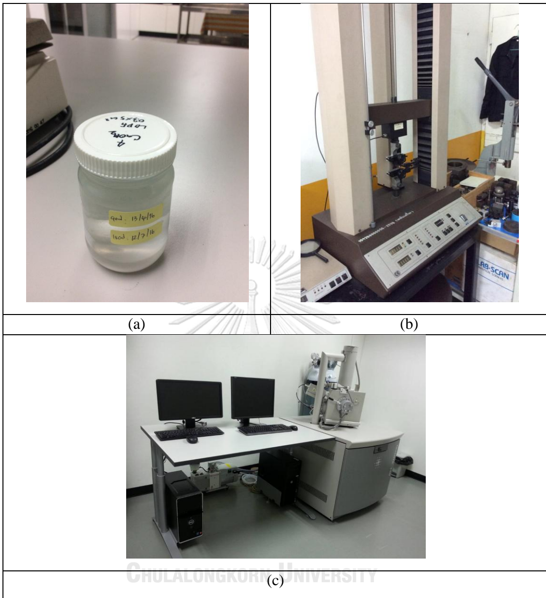
Figure 3.6 Photographs of alkalinity experiment (a) Lime-saturated water in container with plastic fibers, (b) Tensile strength test by 10kN UTM, and (c) Surface analysis by SEM
