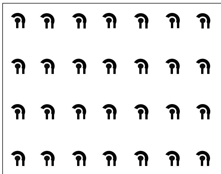
Figure 3.3 The pattern of the blocking stencil for screen-printing by carbon ink.
