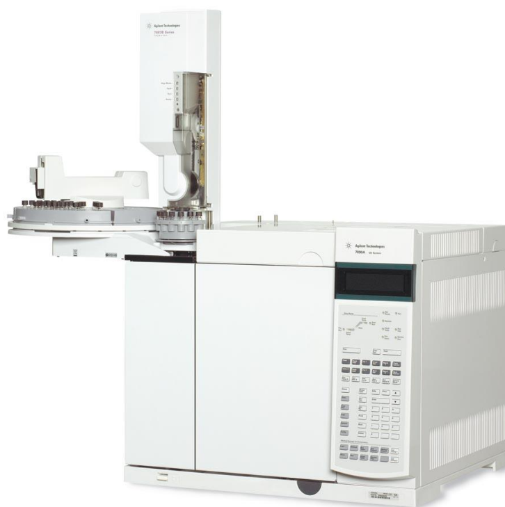
Figure 3.11 GC Agilent Technologies 7890A GC system equipped with DB-5 HT column.
