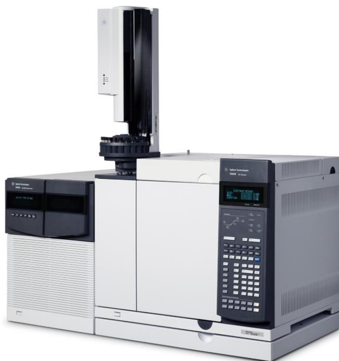
Figure 3.12 GC Agilent Technologies 7890B GC-MS system equipped with HP-5 column.
