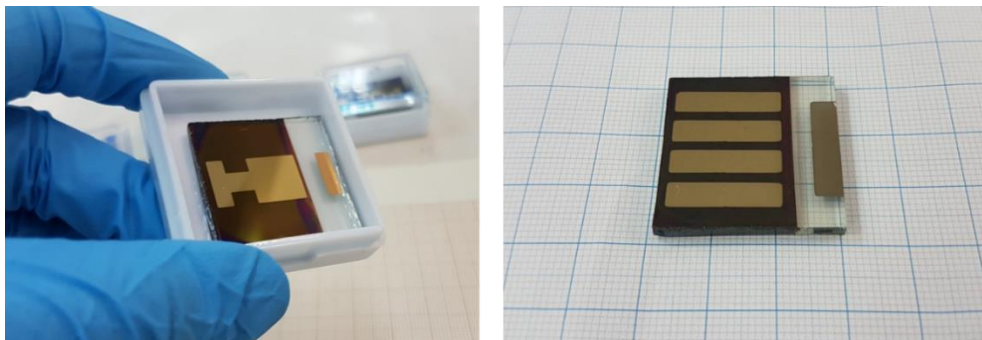
Figure 37 Photographs of complete PSCs with TiO 2 from (a) sputtering and (b) spin-coating methods.
