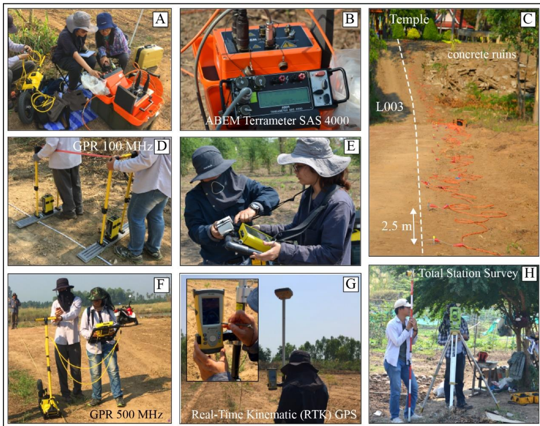
Figure 5.3 Photos of field survey; (A and B) Electric Resistivity survey using ABEM Terrameter SAS 4000, C) Dipole-Dipole array along the L003 survey line, (D, E and F) GPR survey using pulse EKKO PRO instrument, G) Real-Time Kinematic GPS recording positions along the survey lines, and H) Total Station survey.
