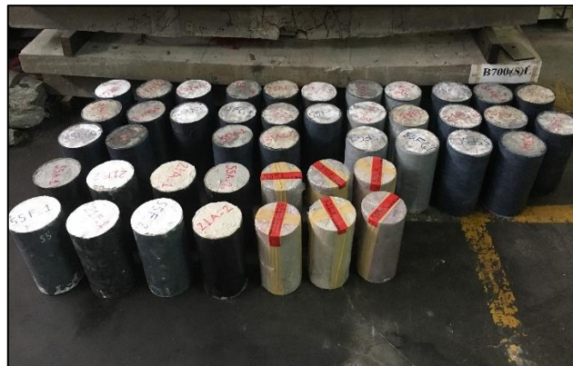
Figure 4.19 FRP wrap curing at the room temperature condition
