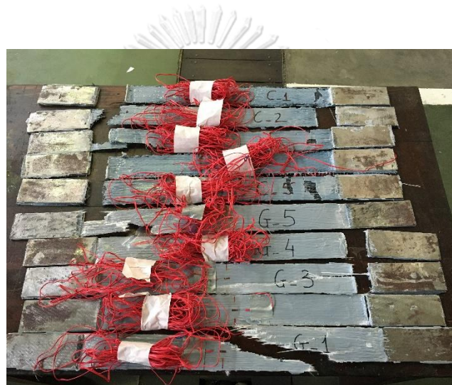
Figure C-3 FRP Coupon's test failure modes
