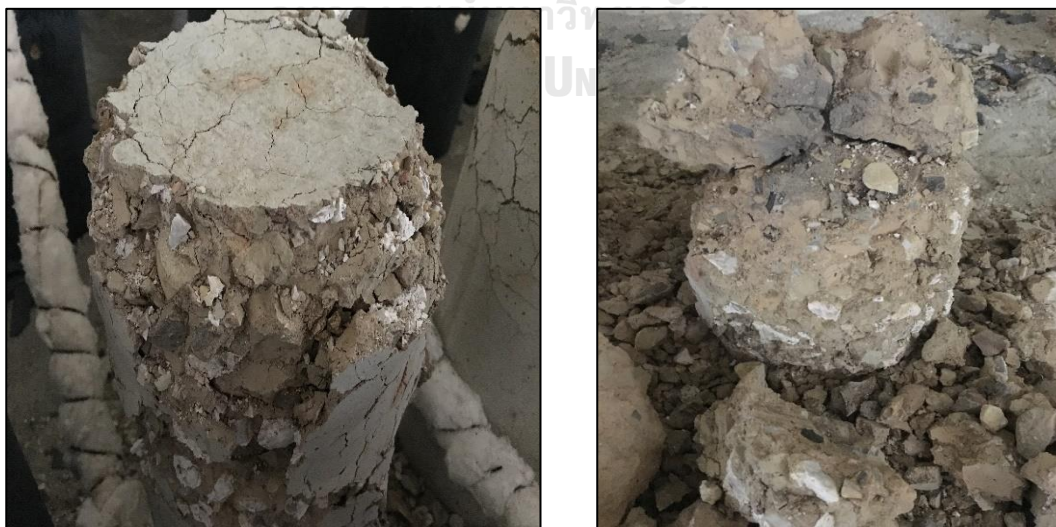
Figure 4.11 Post-heated plain HSC cylinder
