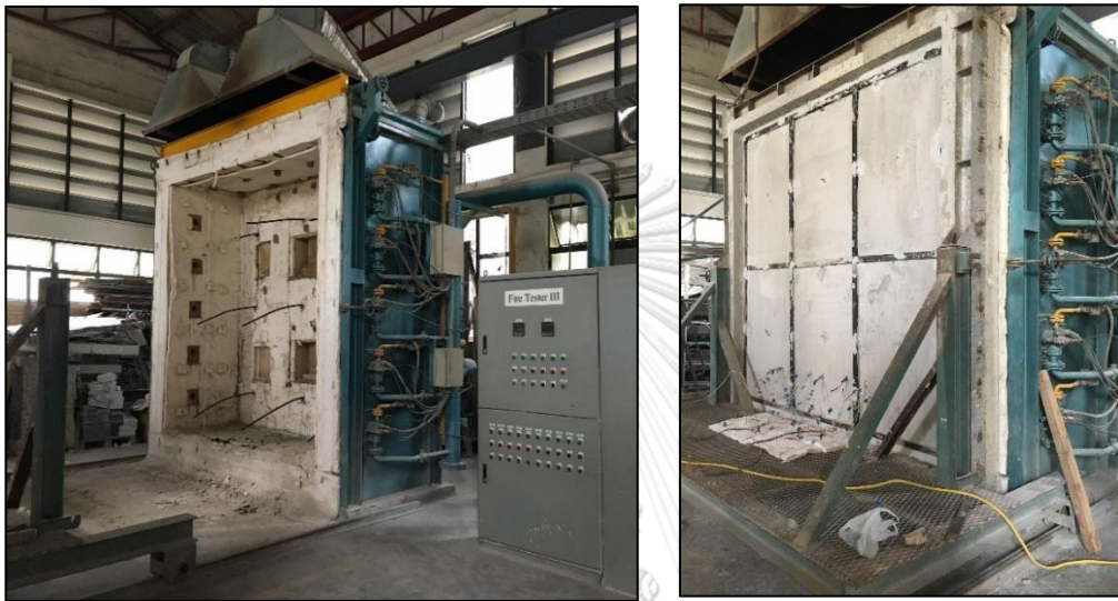
Figure 4.8 Fire furnace at the FSRC, Chulalongkorn University
