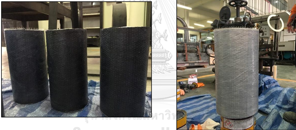
Figure 4.18 FRP-confined CFST columns (fire-damaged and un-fire-damaged)
