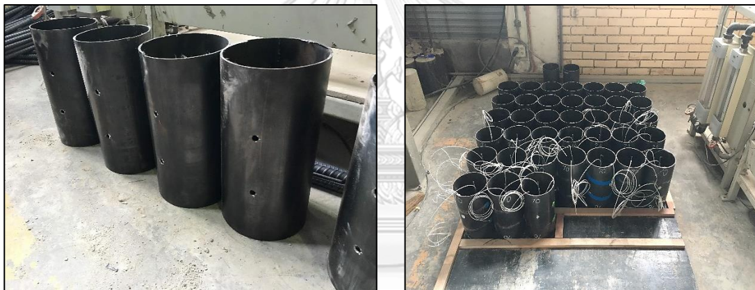
Figure 4.3 Steel tube vent holes and Thermocouples set up
