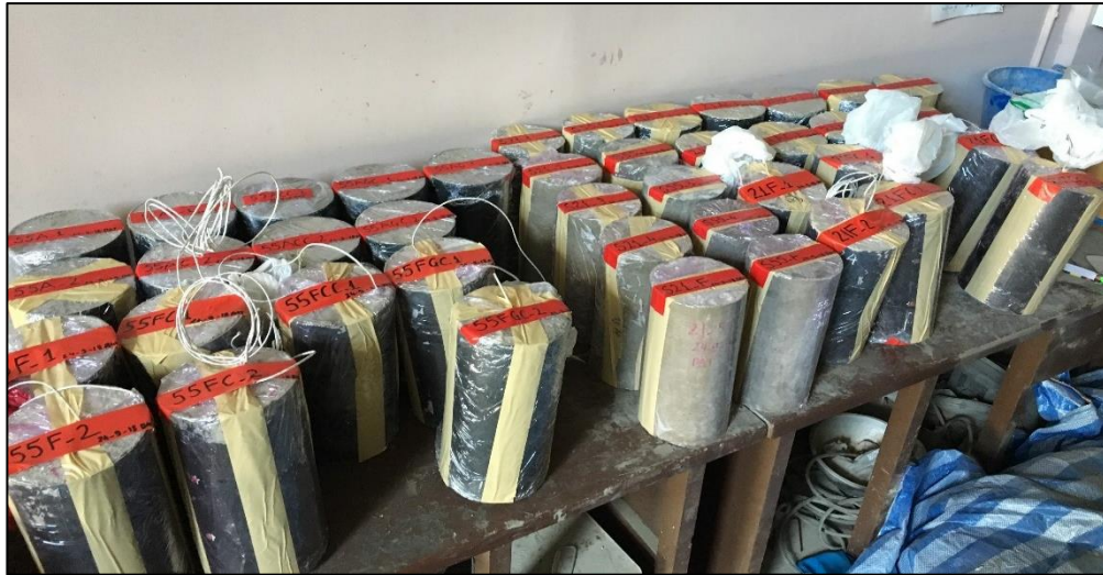
Figure 4.5 Plastic sheet curing and specimen label marking
