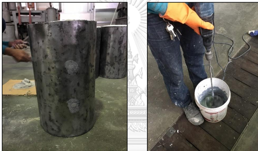
Figure 4.16 Prepared tube surface and adhesive mixing
