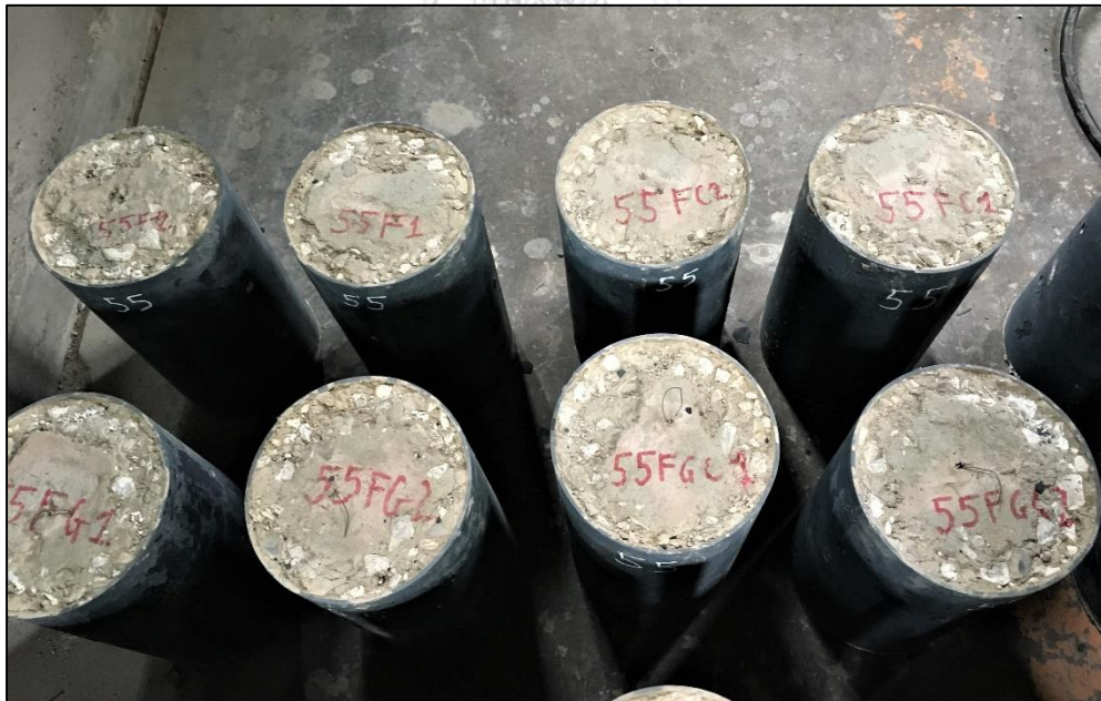
Figure 4.13 Top concrete and steel surface cleaned
