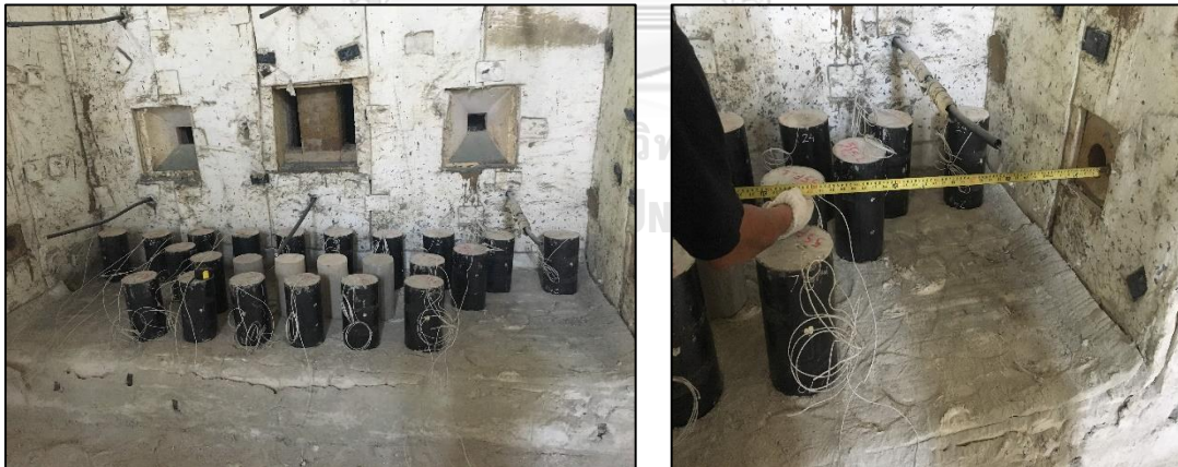
Figure 4.9 Specimen arrangements inside the fire furnace
