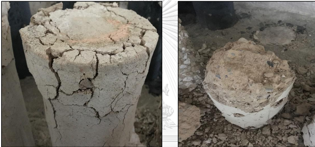
Figure 4.10 Post-heated plain NSC cylinder
