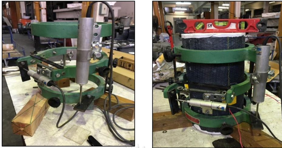
Figure 4.22 Axial, transverse LVDTs set up by Compressometer (ASTM C469)
