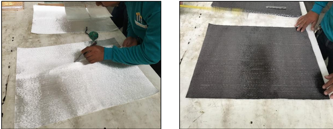
Figure 4.15 GFRP and CFRP sheets cut as designed size (300 x 670 mm)
