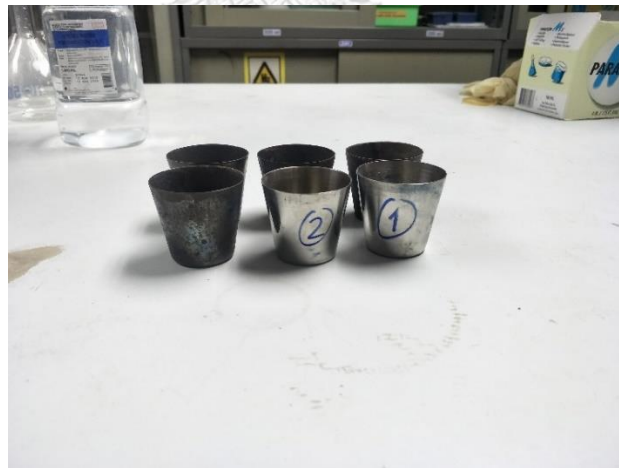
Figure 3.18 The containers used to determine moisture contents
