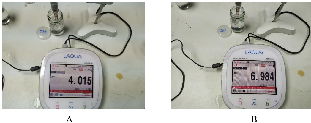
Figure 3.6 Calibrated pH meter by using buffer pH 4 (A) and buffer pH 7 (B)
