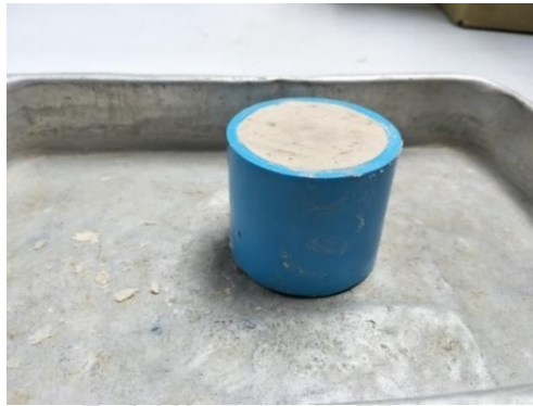
Figure 3.23 Bulk density ring with intact soil core inside
