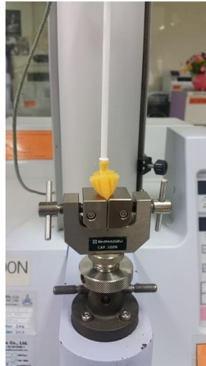
Figure 9 The picture of sponge brush sample clamped in grip for dislodgement of sponge head test.
