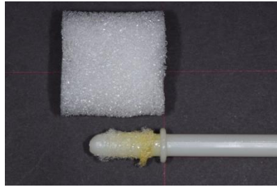
Figure 15 The white sponge head with round shape in cross-section showed a total dislodgement of foam.
