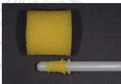
Figure 13 The yellow sponge head with round shape in cross-section showed a total dislodgement of foam.
