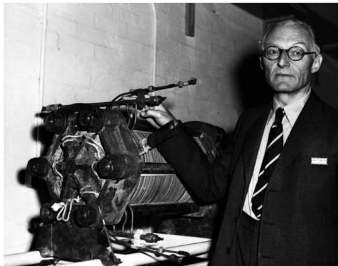
Figure 2. 2 A 6-kW fuel cell developed by Francis Bacon in 1959. [2]
