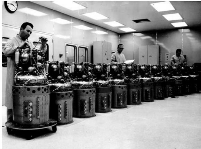
Figure 2. 3 Alkaline fuel cell system for Apollo spacecraft developed by United Technologies Corp. (UTC). [2]
