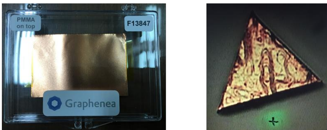
Figure 8-2 (Left) CVD SLG on Cu foil from Graphenea, and (Right) Cut sample magnified by the microscope.
