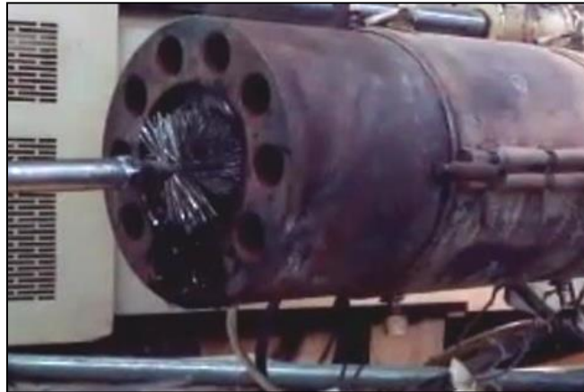
Figure 5-3: Cleaning barrel by using barrel brush
