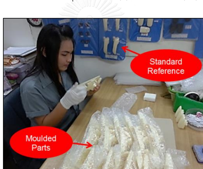
Figure 4-1: Direct visual inspection
