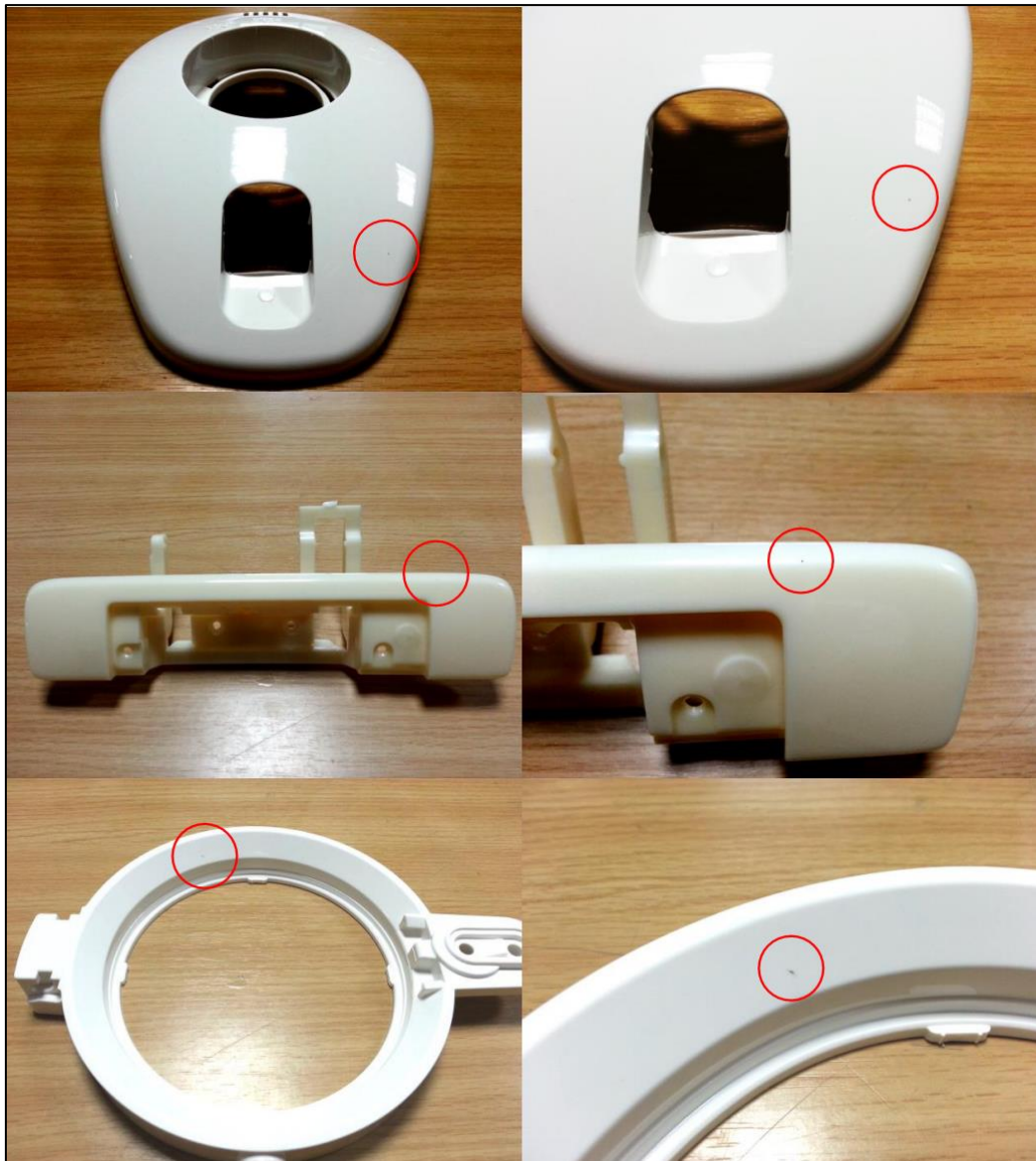
Figure 3-14: Sample of black dot moulded defect parts
