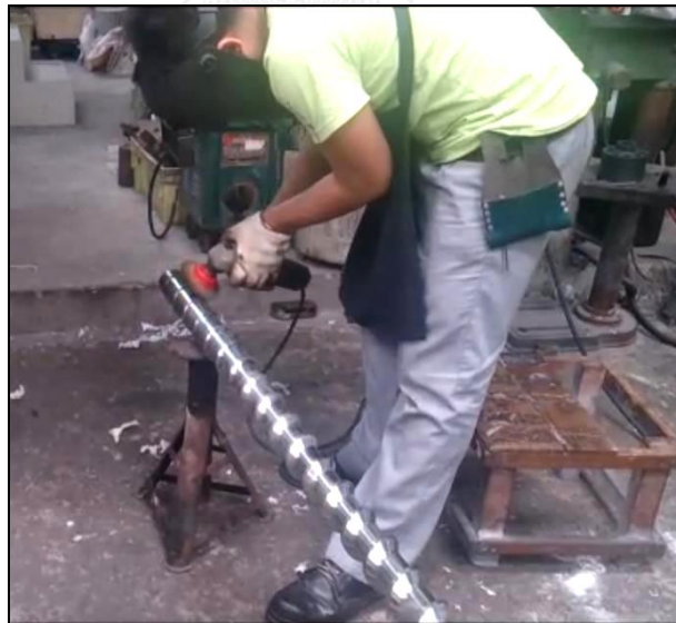
Figure 5-4: Cleaning screw by polishing
