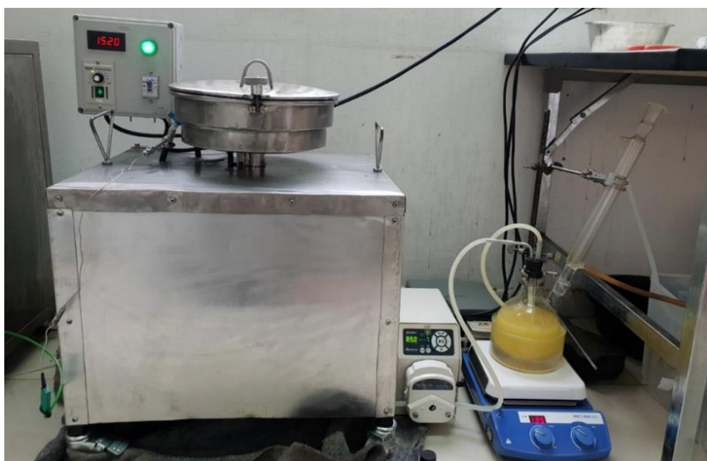
Figure 13 Set up of the RPB-MS reactor.
