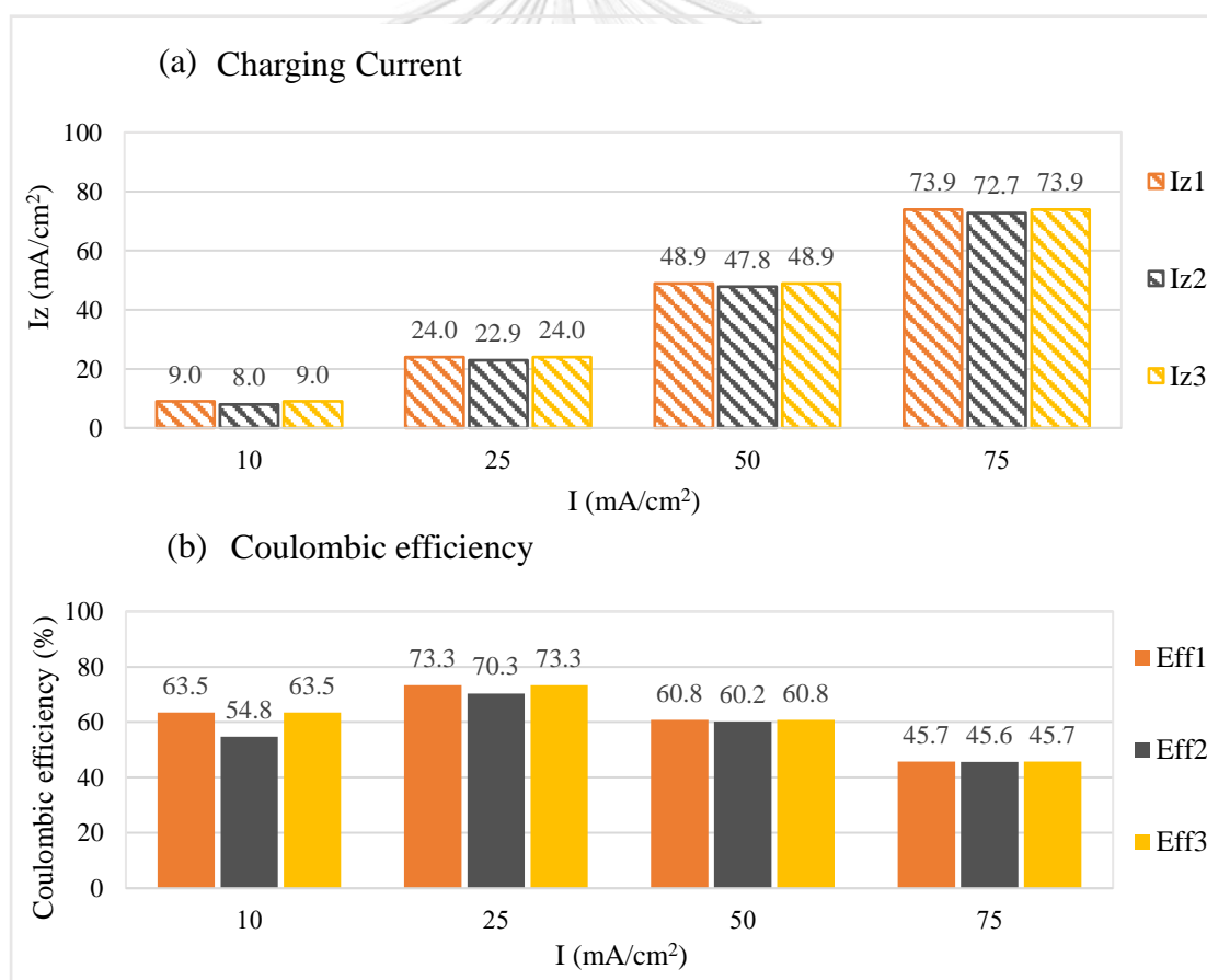
Figure 4.20 The simulation data of charging process which comparing (a) charging current and (b) coulombic efficiency at flow rate 2.5 cm/s as a function of applied current density
