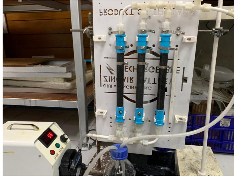
Figure 3.4 The experiment of 3-cells with flowing electrolyte
