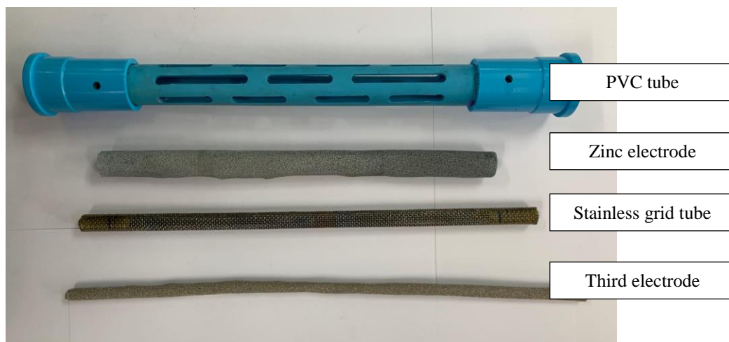
Figure 3.2 The real component of tube zinc-air flow battery
