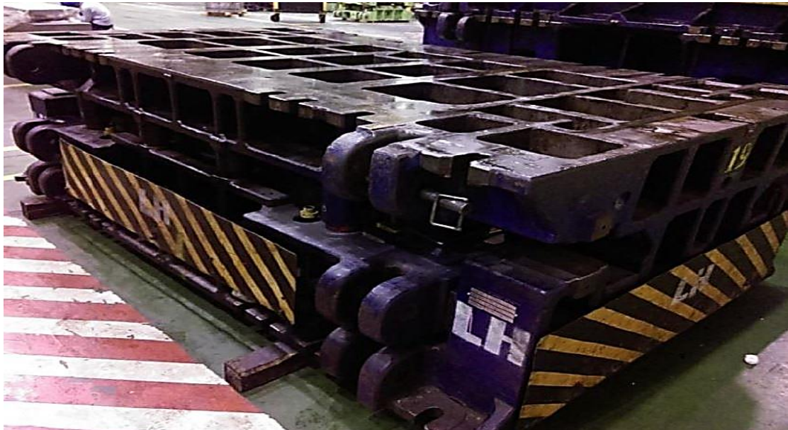
Figure 5.6. New re-strike stamping die.
