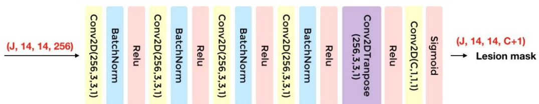
Figure 9: The illustration of the mask frontend for mask prediction in instance segmentation task.
