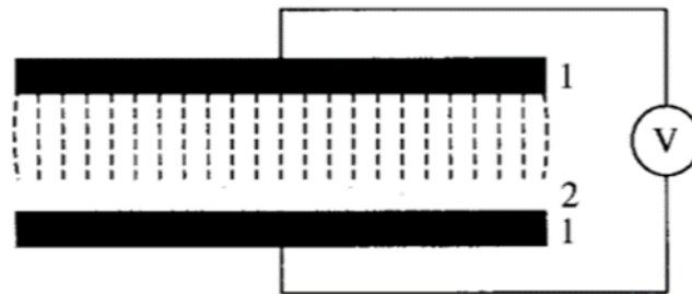
Figure 2.6 Schematic of dielectric barrier discharge ; (1) metallic electrodes and (2) dielectric barrier coating.
