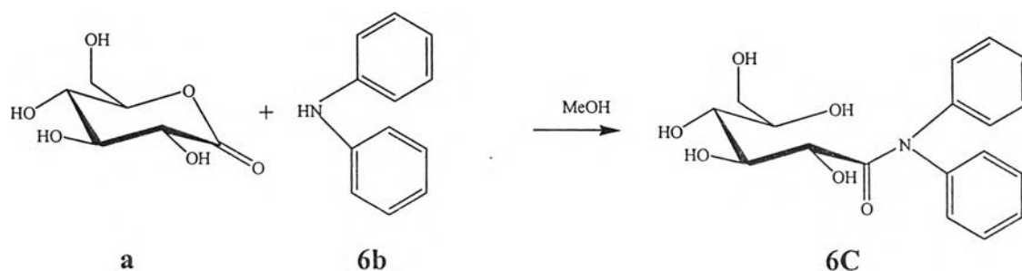
Scheme 3.6 General procedure for the synthesis of N,N -diphenyl–D-gluconamide (6C)
