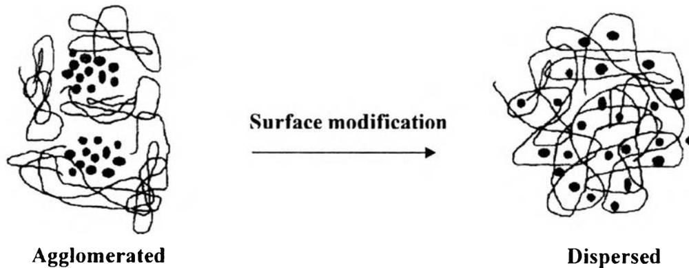
**Figure 2.11** Agglomeration and dispersion of ceramic particles into polymer matrix (Liang *et al.*, 1998).
