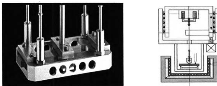
Figure 3.4 : A DMA schematic of dual cantilever.
