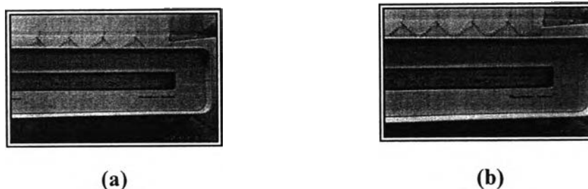
Figure 6.6 Piezoelectric of flat PVDF films shown (a) non-stretching and (b) after stretching at 50 kV/mm.
