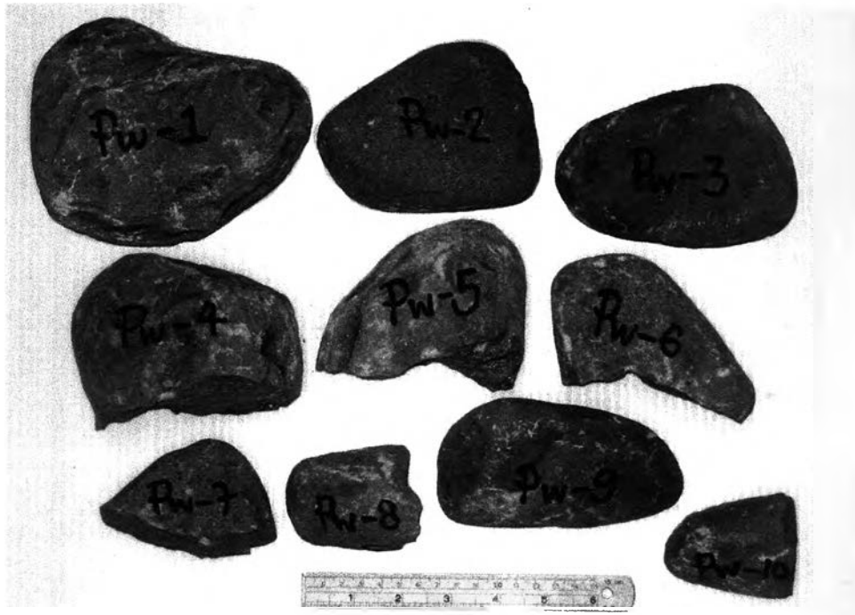
Appendix B-5 Characteristics of ten rock specimens of Phra Wihan sandstone/siltstone (lithologic unit Pw) before point load testing
