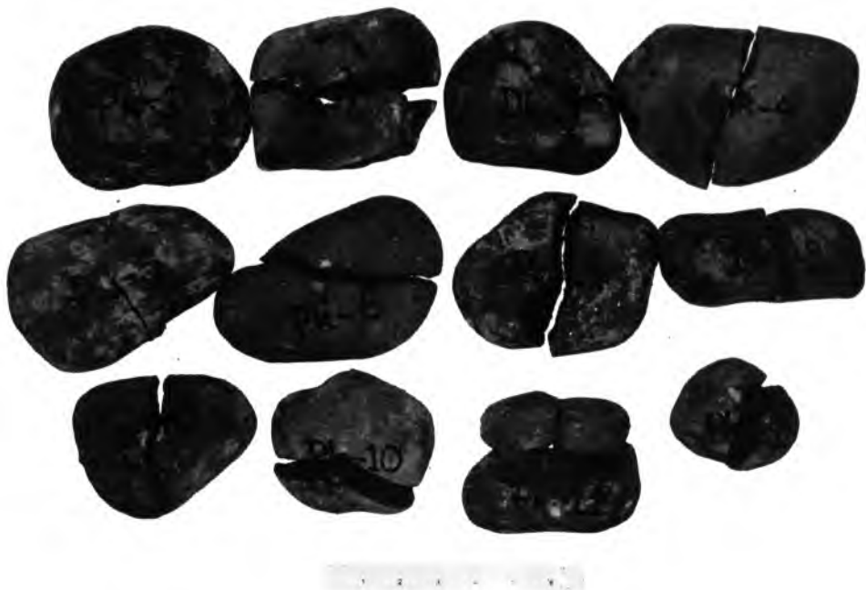
Appendix B-8 Characteristics of twelve rock specimens of Phu Kradung sandstone/siltstone (lithologic unit Pk) after point load testing
