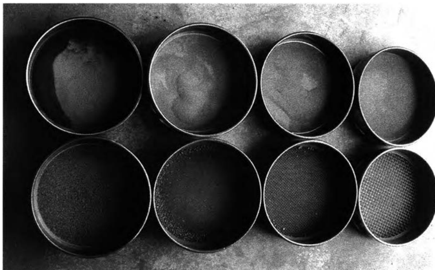
Appendix C-2 Retained soils from each sieve class
